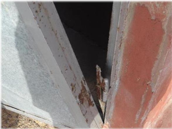
Photo 17 and 18. Degradations observed on the fish smoking kilns: i) the door no longer closes appropriately as a result of the rusting of the hinges; and ii) rust in the drawers.
